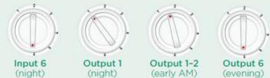
Typical settings for a household which is out during the day and needing heat in the evening
