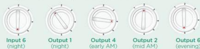
Typical settings for a household needing heat during the day and needing heat during the evening
